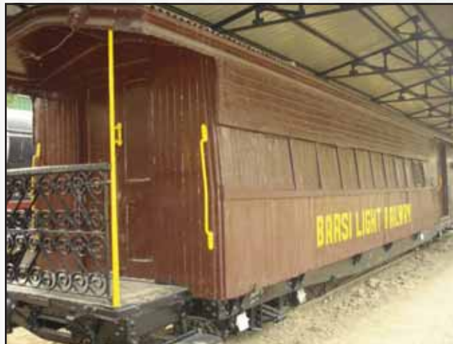
High capacity wooden bodied coach with steel under-frame.
