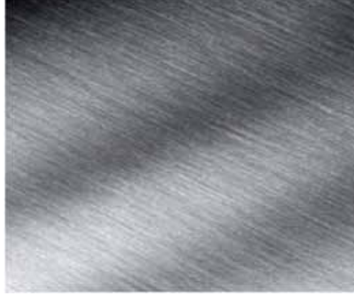
Matt Finish Grit 120 0.8 micron Ra (Surface roughness)
