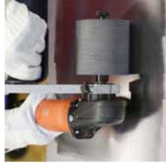
Sanding sleeve of Grit 180 with 900 rpm
