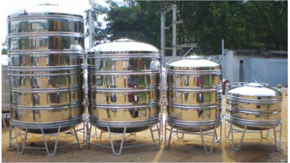
water to be heated up during the day and it cools faster during evenings and night because of high thermal conductivity. The detailed results can be analyzed from the graph which states that even in the case of different surface finish SS tanks performs better than plastic tanks.
