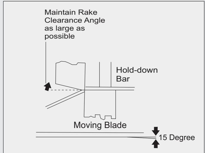
The most suitable shear blades for cutting 409M and stainless steel are made of high carbon – high chromium tool steel. The blades must be kept sharp – a good test is to cut a piece of paper.
