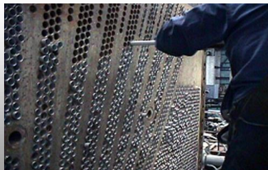
Heat exchanger tubes in UNS S44660 for a seawater condenser. Courtesy Plymouth Tube
