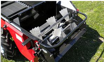
Martensitic stainless steel beater bars in a manure spreader
