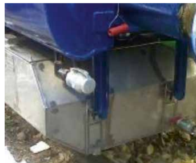
▲ A stainless steel bio-digester tank flitted.
