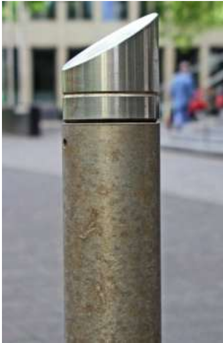
Type 316 Bollard Dusseldorf Rough bottom finish Deicing salt
