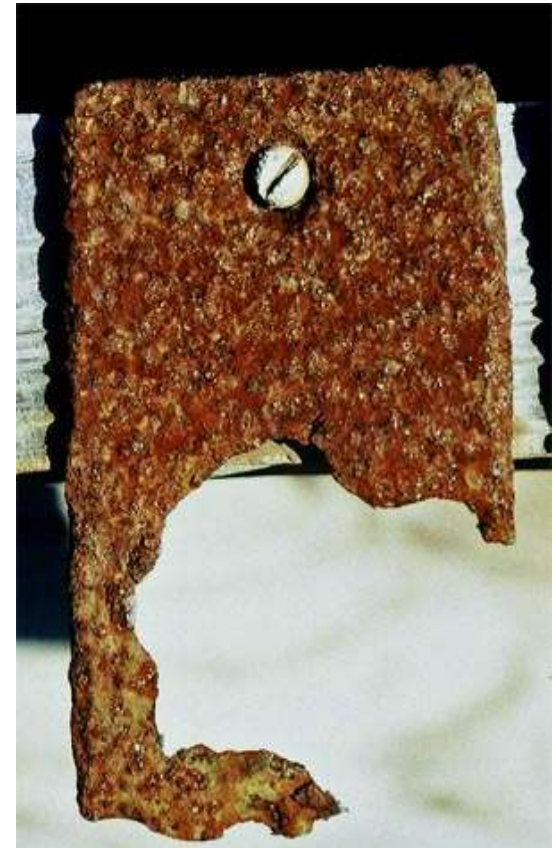
Carbon steel 60 Zn, 20 Al, 20 Mg coating 9
