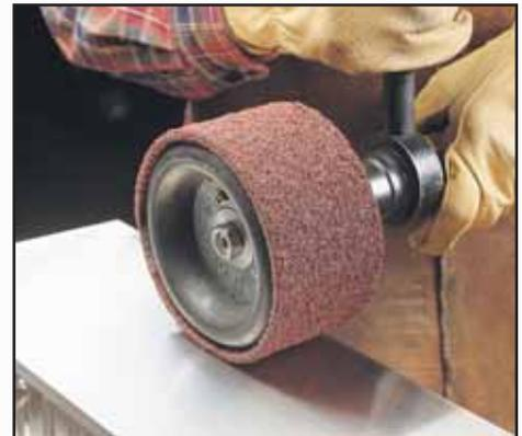
Different combinations of above products helps achieve different hairline or matt finishes and even helps restore the finish post the fabrication process. The process of finish generation includes 4 simple steps – weld grinding, blending, setting the grain, and final finishing. Using the above process sequence and choosing the right abrasive and tool helps achieve the desired finish.
